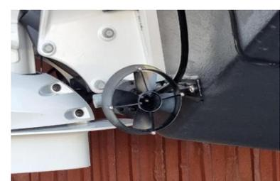
**Engine:** 2600w 3-phase direct-drive water-cooled.
