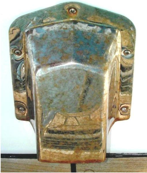
Stainless steel do also needs maintenance to keep nice and shiny. Brown spots can occur on stainless steel parts that are in contact with salt water, especially stainless steel anchor equipment that are exposed for extreme environment.
