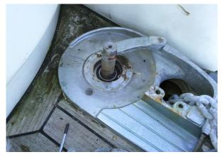
When disassembly the gear motor and the shaft is stuck in the gear box, this is how you can disassembly from deck side. Shaft get stuck if the installer has forgot to put grease on shaft when installing, or lack of maintenance
